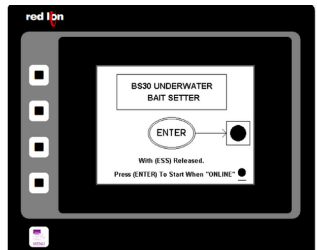
Figure 6.8. Confirmation of action on reset screen of deck service box.
