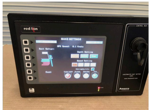
Figure 2.6. Make settings screen on the control box
