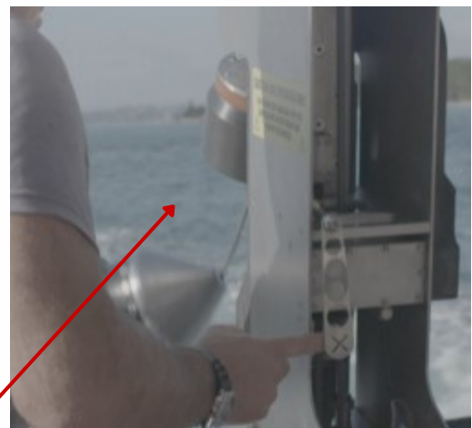
Figure 4.4. Keep hands clear of the area between the capsule and nose cone (indicated by the blue arrow).
