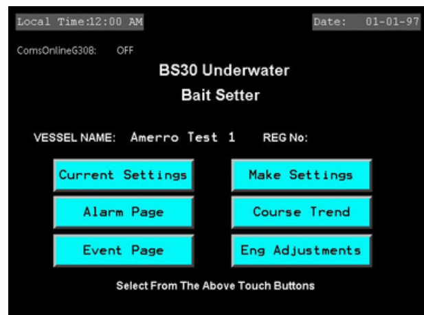
Figure 6.3. The menu screen on the control box.
